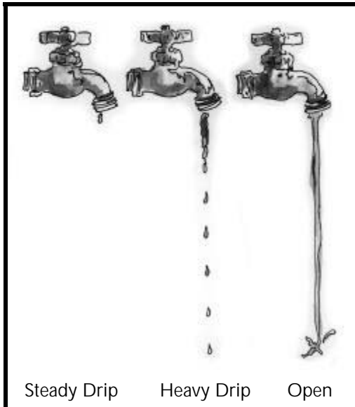
Figure 3.3 A slow steady leak (i.e., one drop per second) from a faucet may create a water loss of 36 gallons per day. A heavy leak may lose 180 gallons per day. A fully open faucet flowing at 2.5 gallons per minute will pour out 3600 gallons per day.
