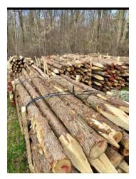
Pictured at left are cedar fence posts which can be obtained for \$16 per post. Peeled posts can be obtained for \$20 per post. A lift of 100 posts for \$1900 can be delivered at no additional cost. Posts will be trimmed to use as trusses for bridges and ripped down to 1" thickness to serve as bridge decking of varying width and secured with 3" T25 decking screws. Screws are \$60 per 5lb bucket from Douglas Lumber.
